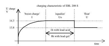
If due to high loads the 13.8V floating voltage can't be provided the battery charger switches over from float to boost-charge after a delay of approx. 5 sec.
